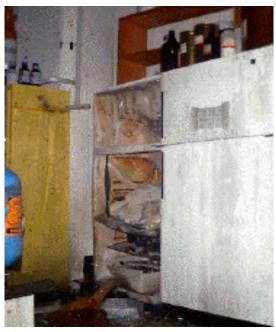
Thermostat inside, left side, caused spark.
