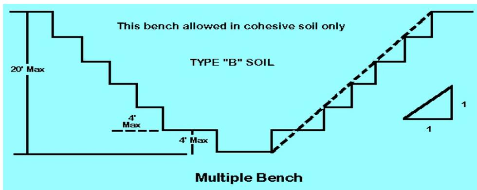
In Type B soil, the vertical height of the benches must not exceed 4 feet. Benches must be below the maximum allowable slope for that soil type. In other words, a 10-foot deep trench in Type B soil must be benched back 10 feet in each direction, with the maximum of a 45-degree angle.
