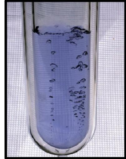
1. If the liquid nitrogen dewar is removed and the remaining liquid has a blue color (or if any liquid is observed), assume liquid oxygen is present.
